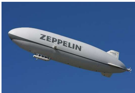
Fig. 1. Airships can be filled with either hydrogen or helium gas. Although hydrogen is lighter and produces more lift, helium is preferred for safety reasons (hydrogen being flammable).
